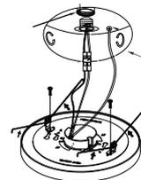
**Step 3:** Connect quick connectors and tuck all wires into recessed can. Squeeze springs and push up into recessed can.
