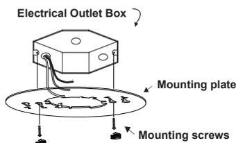
**Step 2:** Connect supply wires to wires on the fixture with wire nuts, or push wires into Quick Connector. Connect white to white, black to black, and copper wire to copper wire as grounding connection.
